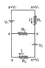
$$\frac{V_1}{R_1} = \frac{V_2}{R_3}$$
