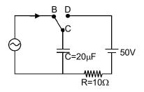
Final charge on capacitor =  $20 \times 10^{-6} \times 50 = 10^{-3}$  C (Upper plate positive)
